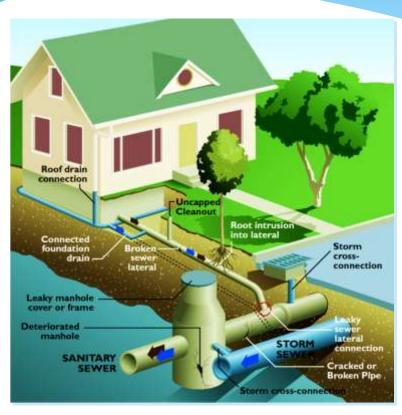
This graphic shows the ways that stormwater runoff can get into the sanitary sewer system. In some cases, it seeps in through breaks in the pipes. However, in other cases it gets in through deliberate connections that channel the stormwater runoff into the sanitary sewer system.
